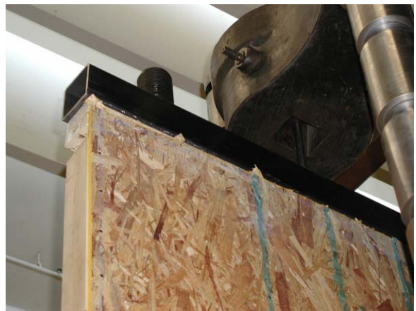
Figure 9 - Sheathing nails along top plate failure (T4)
