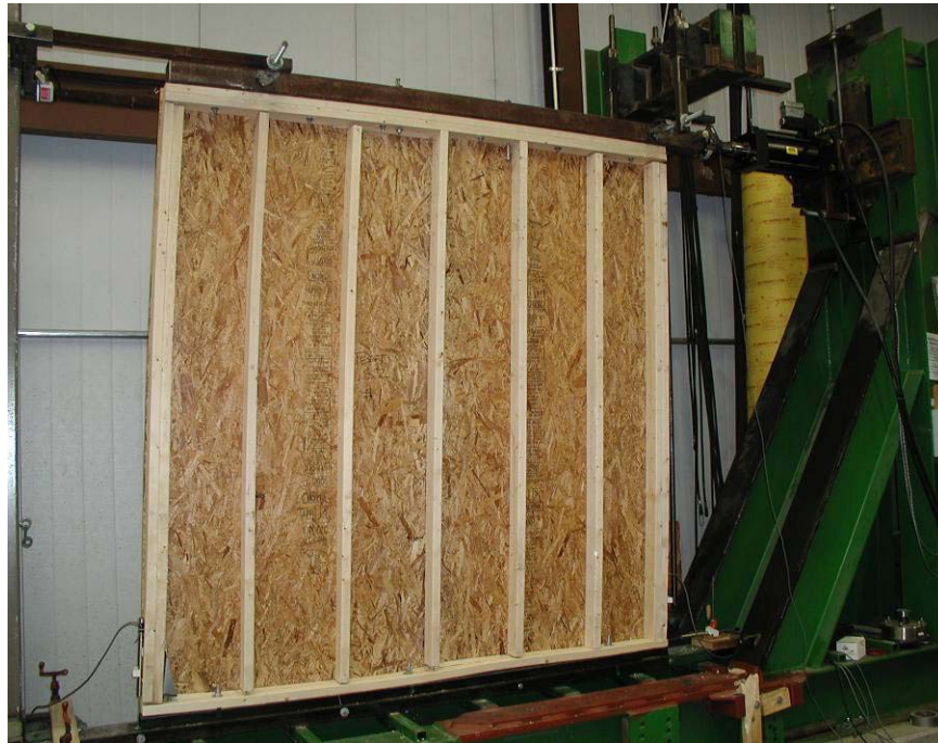
Figure 4 - Photograph of Shear Wall Test Setup
