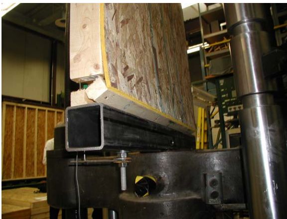
Figure 8 - Cross grain bending failure (T3)
