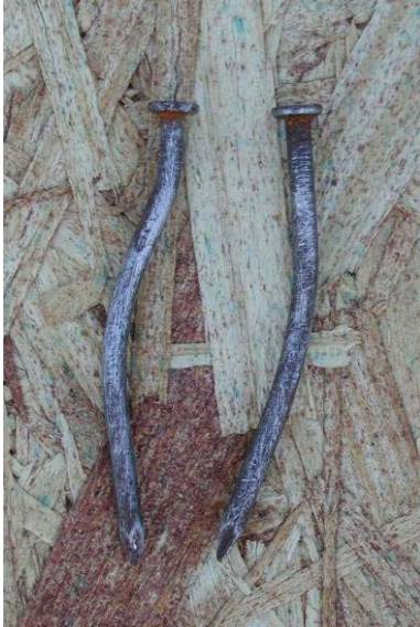
Nails from the bottom plates of specimens T4-1 and T4-3
