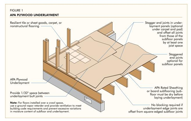
One of the keys to good performance in floors is the right combination of subfloor, underlayment and finish flooring. Plywood Underlayment panels provide a smooth base for carpet, tile or sheet flooring and other types of finish flooring. APA Underlayment also resists dents and punctures from concentrated loads.
